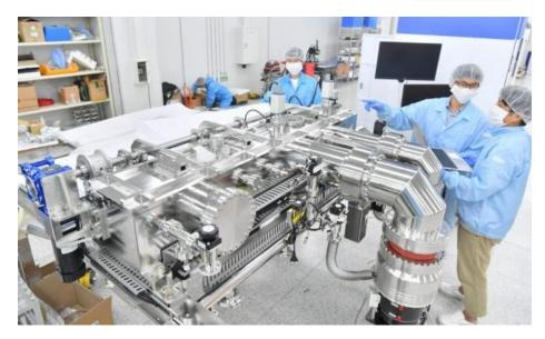
Researchers are manufacturing the main chamber part of the EUV light source in the clean room at ESOL, an EUV equipment company located in Dongtan Industrial Complex, Hwaseong-si, Gyeonggi-do.
