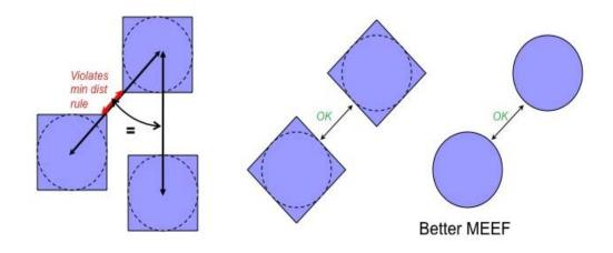
Figure 1. Using circles on the mask for vias and contacts benefits both design density and manufacturing tolerances.
