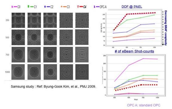
Figure 2. Curvilinear assist features are critical to achieving acceptable DOF at advanced process nodes, but traditional approaches to creating these features can be too costly in terms of write-time.
