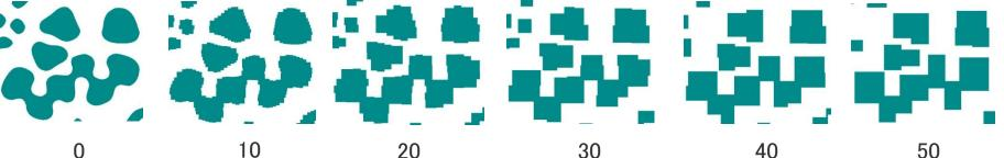
Aggressive Contour Modest Contour For coarser masks printing image degrades and can cause failure of guiding pattern to control positions of DSA cylinders
