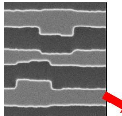
Simulation is able to very accurately simulate the mask shape for VSB ebeam litho
