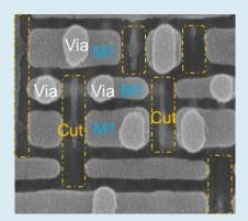
Direct, on-device, in-die measurement
