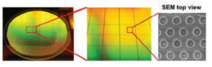
**FIGURE 10.** Full wafer scale imprinted wafer for photonic crystal application.
