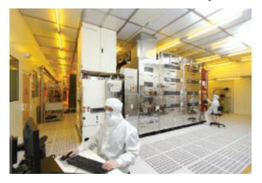
**FIGURE 7.** MAPPER FLX-1200 in Leti cleanroom interfaced with a SCREEN DUO track. Key figures of the tool: Acceleration voltage 5kV; throughput: 1wph with 1,300 beamlines; resolution/alignment specs:  $32nmhp / 10nm 3\sigma$ .
